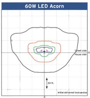
Distribution: type 3 roadway Initial delivered lumens: 7,438 Luminaire mounting height: 13.5 feet
